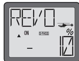
7) Press the SELECT key once again to access the revo mixing adjustments for the high side. The up arrow on the left side of the screen indicates that it is the high side that will be adjusted.
