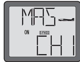
The master channel, as the name suggests, is the channel that will be the controlling channel. The slave channel, which will be determined in the next step, is the channel that will be controlled by the master channel. That is, the slave channel will operate based on input from the master channel.
