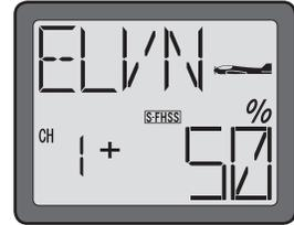
7) Adjust the elevator channel’s travel. Press the SELECT key to display the “CH2” and flashing “%” sign. Use the DATA INPUT lever to set the percentage of rudder travel rate. The values are adjustable from -100% to +100%.
