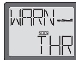
Move the throttle position to the lowest position in order to silence this alarm accordingly.
