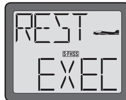
**Note:** If the power switch is turned off while reset is underway, the data may not be reset.
