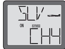
As noted above, the slave channel is the channel that follows the input control based on the rates and input from the master channel.
