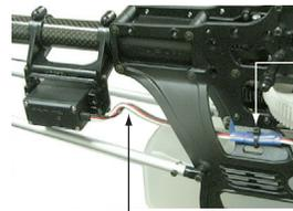
Fasten about 5-10cm from the servo outlet so that the lead wire is neat.
