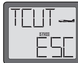
6) Momentarily press and hold the throttle-cut (THR CUT) button on the left side of the transmitter. The electronic speed control in the model will be disarmed.
